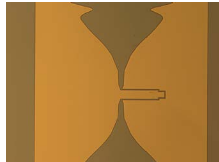
Figure 2: Fabricated bowtie aperture antenna with CPW feed.
