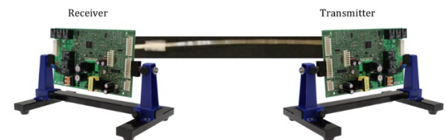
Figure 3. Conceptual diagram of dielectric waveguide demonstration set up.
