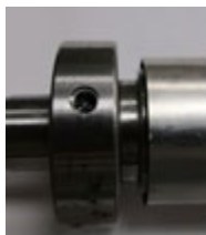
Figure 1. Outer race fault in bearing of test motor.
