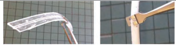
Figure 2: Flexible PDMS nano-composite waveguides. a) No \text{TiO}_2 . b) 5% \text{TiO}_2 by weight.
