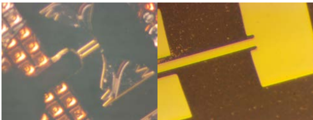
Figure 1: (Left) 180-300 GHz hybrid CPW fed modified bowtie antenna with probe; (Right) 280 GHz microstrip patch
