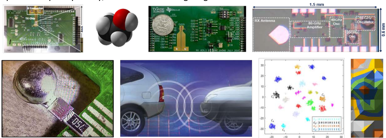
Figure 3. (Top left) 200-260 GHz CMOS transmitter and receiver for rotational spectroscopy (K. O. W. Choi, UT-Dallas), (Top right) Injection-locked receiver for synchronization of widely spaced imaging array (A. Babakhani, Rice U.), (Bottom left) Vibration sensor compatible with conventional silicon IC and packaging technologies (S. Pourkamali, UT Dallas), (Bottom left center) Automotive radar imaging (M. Torlak, UT-Dallas), (Bottom right center) Projected e-test space, where each point represents a wafer. A proper test flow to each process signature of each wafer is assigned to maximize the test cost reduction while maintaining the test escape rate below a target level. (Y. Makris, UT-Dallas), (Bottom right) Magnitude of field inside a dielectric waveguide (D. MacFarlane, SMU).
