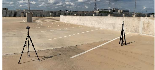
Figure 1. Open space BLE measurement environment with a TI CC26X2R1 multi-antenna board mounted on each tripod.
