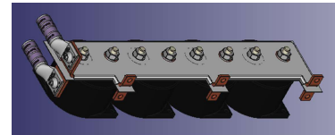
Figure 3. 3D view of the inverter busbar for 400A and 1100V.
