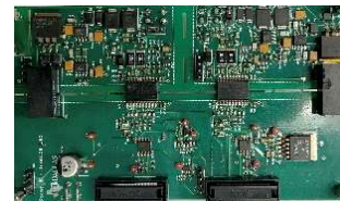
Figure 1. The gate driver board with embedded condition monitoring systems for different aging mechanisms.
