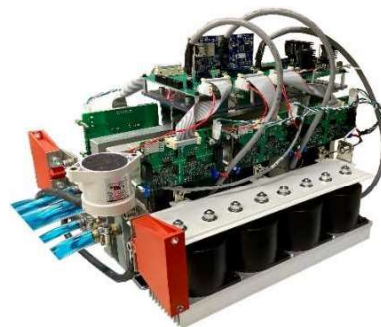
Figure 3. AC power cycling test setup.
