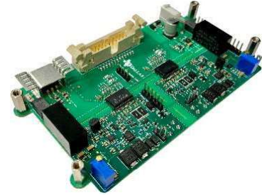
Figure 1. Second version of gate driver board with embedded condition monitoring systems for different aging mechanisms.
