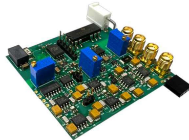
Figure 2. Transconductance daughter Board.
